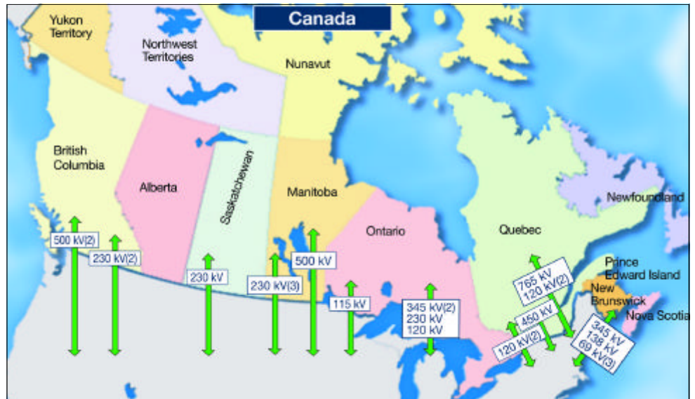
Note: The numbers indicate the voltage of the power lines from each province to the states. If there is more than one line with a given voltage, the number of lines is indicated in parentheses.
