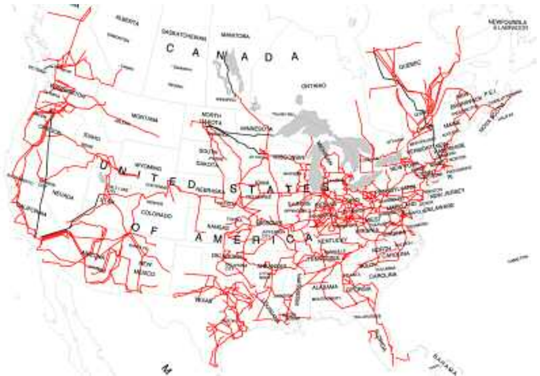
Map copyright CEA. Lines shown are 345Kv and above. There are numerous interconnections between Canada and the U.S. under 345Kv that do not appear on this map.
