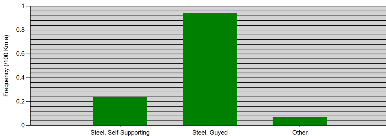
Frequency of line-related sustained forced outages of 500 - 599 kV transmission lines by supporting structure.
