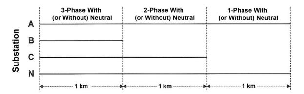
Total Circuit Length = 3-Ø + 2-Ø + 1-Ø = 1 km + 1 km + 2 km = 3 km Circuit Length
