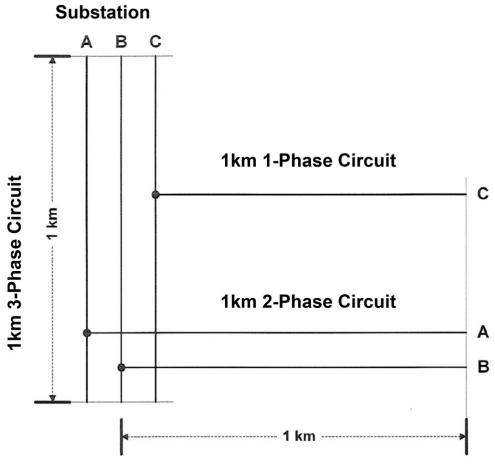
Total Circuit Length = 3 - Phase + 2-Phase + 1- Phase = 1 km + 1 km = 3 km Circuit Length
