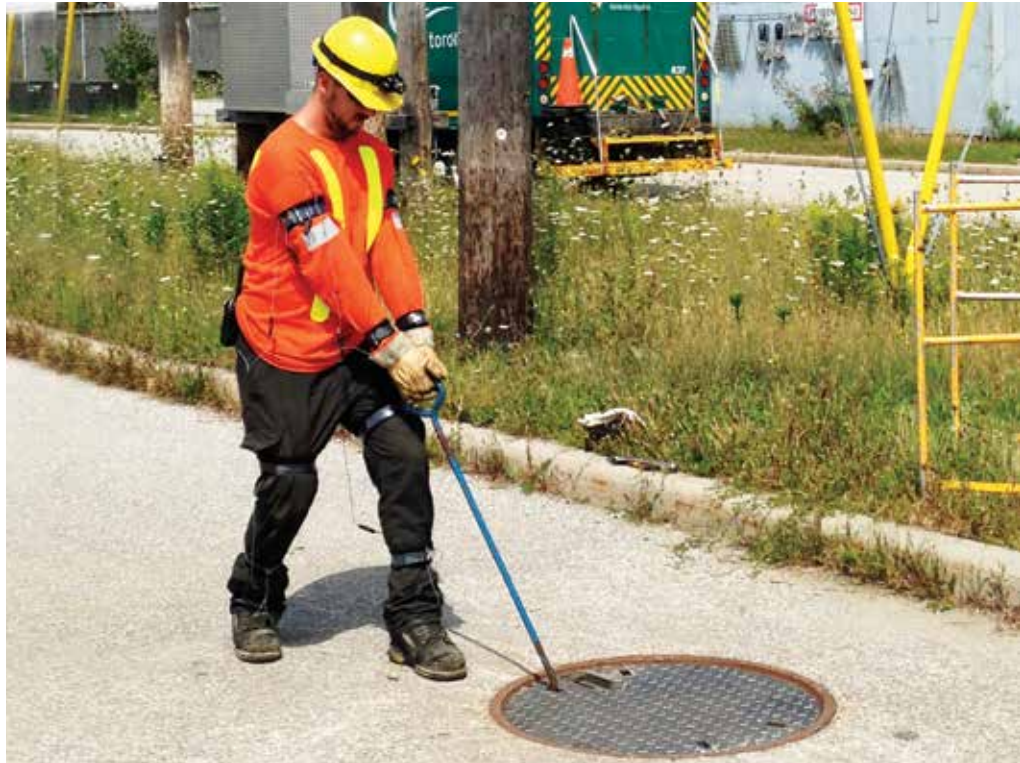
Toronto Hydro employee is outfitted with the IGS-180i motion capture suit built by Animazoo. The suit includes 11 sensors placed on the trunk and limbs of the participant, which are used to create a digital record of the participant's movements while lifting the chamber lids with the different tools. This data can then be used in a simulation program to determine the joint loading of the shoulder and spine when lifting the chamber lids. Photo courtesy of Toronto Hydro Corporation.
