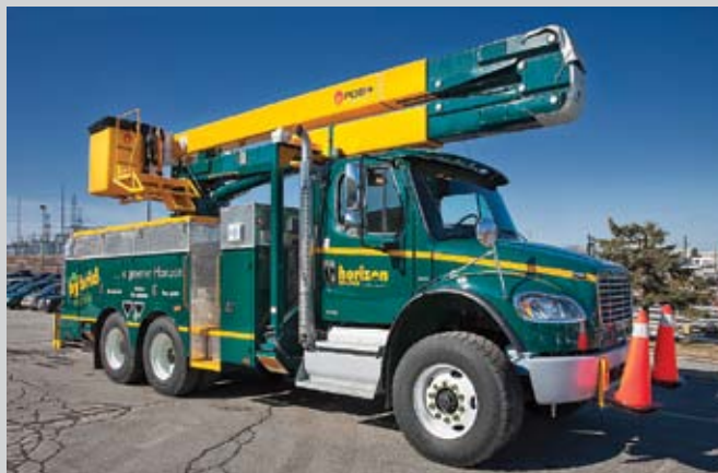
Horizon Utilities' single-bucket hybrid and plug-in combination vehicle purchased in 2010. Hybrid electric vehicles combine conventional and electric propulsion systems to achieve better fuel economy and reduce emissions.
