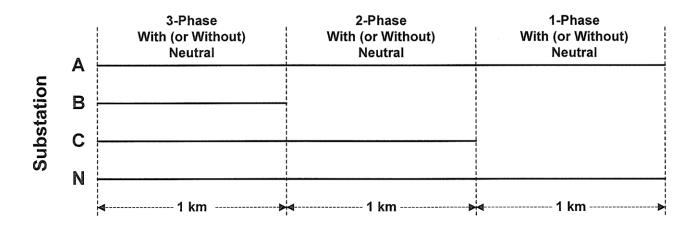
Total Circuit Length = 3-Ø + 2-Ø + 1-Ø = 1 km + 1 km + 1 km = 3 km Circuit Length
