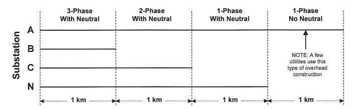
Total Circuit Length = 3-Ø + 2-Ø + 1-Ø = 1 km + 1 km + 2 km = 4 km Circuit Length
