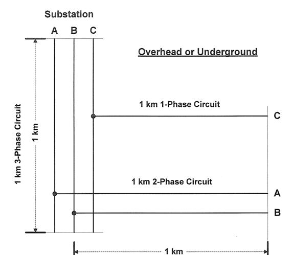
Total Circuit Length = 3-Phase + 2-Phase + 1-Phase = 1 km + 1 km + 1 km = 3 km Circuit Length
