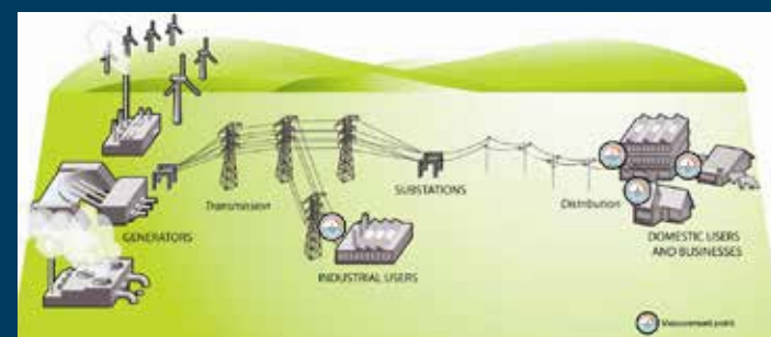
Figure 1: The traditional one-way flow of electricity. Source: Government of New Zealand
